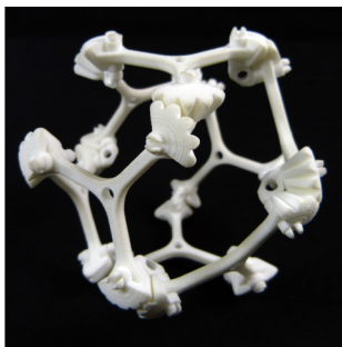
Figure 5 The gears on this version of Buckminster Fuller’s expanding and contracting “jitterbug” mechanism help to keep the parts aligned, making the movement smoother. Joint work with S. Matsumoto.
